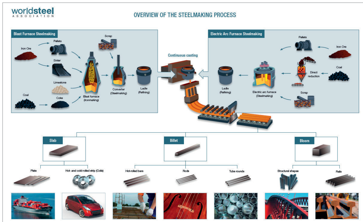
Figure 17.2.1: Overview of the steel making process and variety of products manufactured. [Source: World Steel Association] 92
