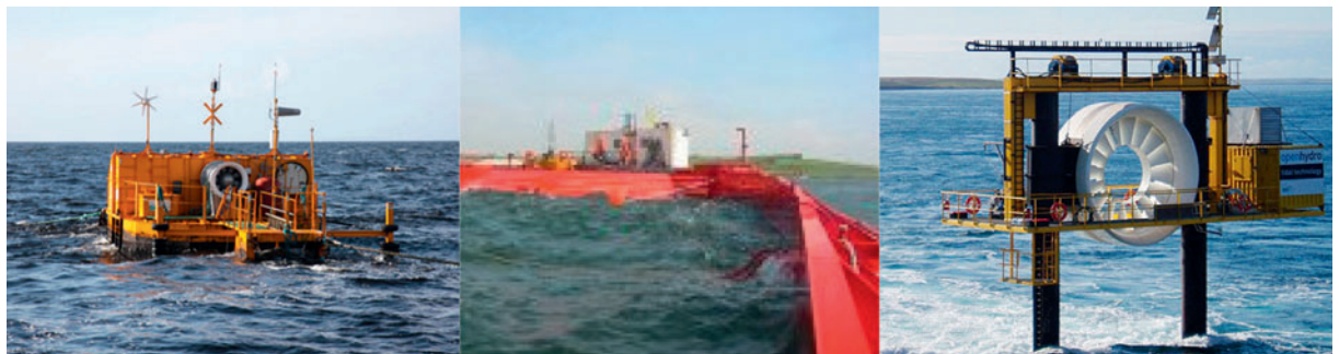
Figure 6.1: Typical marine energy technologies (from left to right): floating OWC, overtopping Wave dragon and Open Hydro (tidal) [Sources (left to right): Ocean Energy Ltd., Wave Dragon Ltd., Open Hydro Ltd.]
