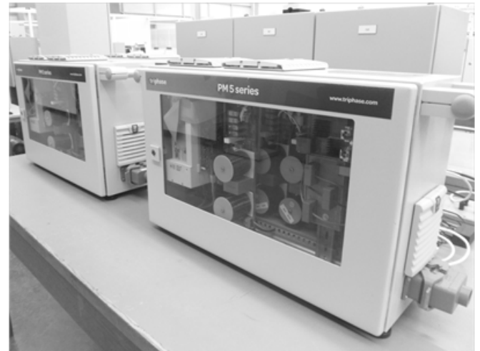
Fig. 6: Two of the three 5kVA AC/DC converters sitting on the laboratory of TU Delft EPP group.
