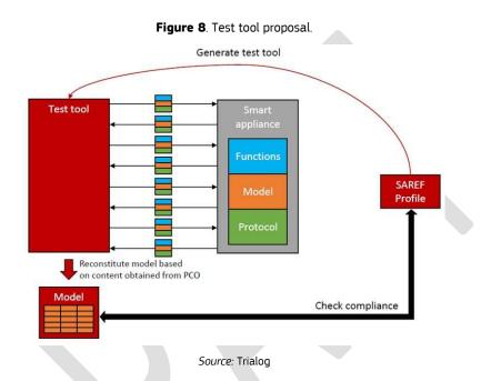
A schematic diagram can be found in Figure 5. The diagram shows the test tool connected to an ESA and performing the check above described. The test tool reconstitutes the model obtained when connected to the ESA and compares it with the correct one, generated previously considering the SAREF triple specifications. The specifications for every UC can be found in Annex 2 of the CoC.
