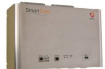
DTC installed in all secondary substations
